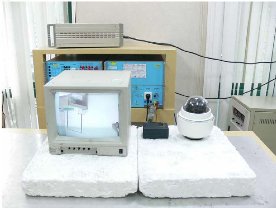
Set Up Photo of EFT AC power line
