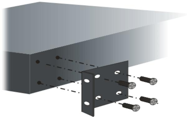
After the bracket installation, the Vigor3910 Series chassis can be installed in a rack by using four screws for each side of the rack.
