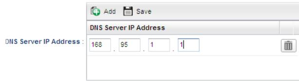
**Save** – After finished the IP address configuration, click Save to save the setting onto the router.
