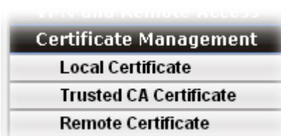
Local certificate is created by the end user and must be signed by a trusted CA center. Vigor2960 can serve as a trusted CA and is called with “Root CA”. Therefore, any user can ask for certificate signed by Vigor2960.
