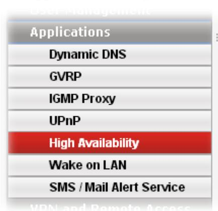
3. In the tab of **High Availability Global Setup**, choose **Hot-Standby** as Redundant Method; choose **Secondary** as Config Synchronization Rule; type the lan1 IP address configured in router A; type **draytek** as Authentication Key; choose **Automatic** as Advance Preemption Mode. Click **Apply** to save the settings.
