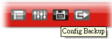
There is one way to store current used settings quickly by clicking the **Config Backup** icon. It allows you to backup current settings as a file. Such configuration file can be restored by using **System Maintenance>>Configuration Backup**.
